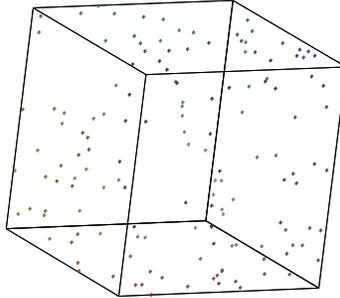
Like any measurement, the coordinates contain errors, but the engineer can take points that lie on a plane, and find, in the *Least Squares* sense, the *plane* of best fit:  $z = ax + by + c$ . The *normal equations* will be given by three equations in three unknowns.
